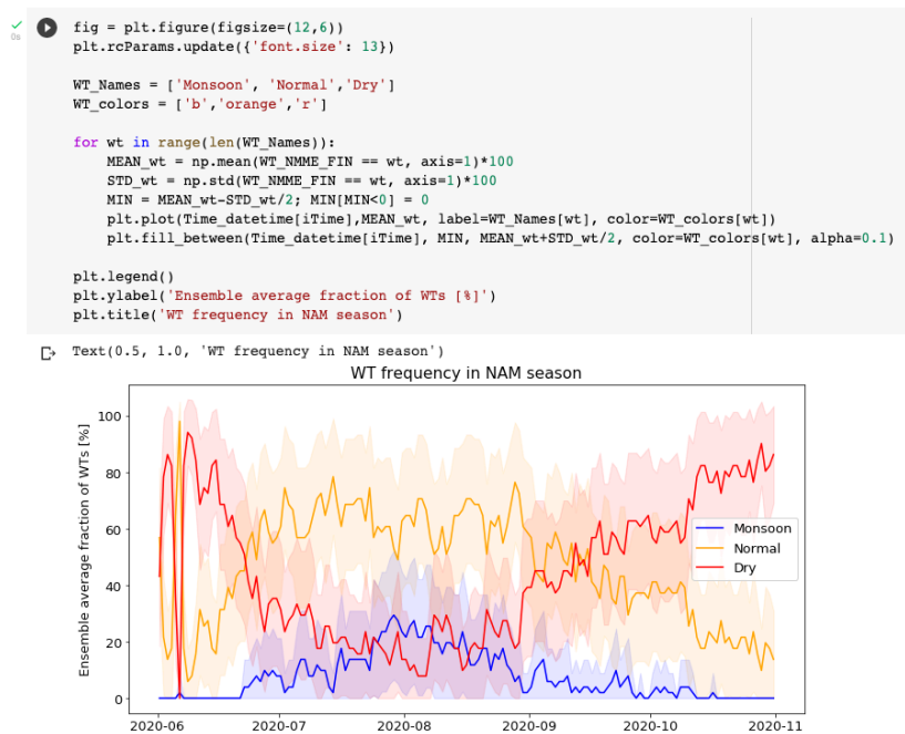
Figure 7. The Google Colab Notebook plots the ensemble mean WT frequency for June through October of 2020.
